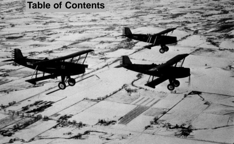
Front Range formation: Acquired in 1928, the unit's Douglas O-2Hs had difficulty flying at high altitudes.
