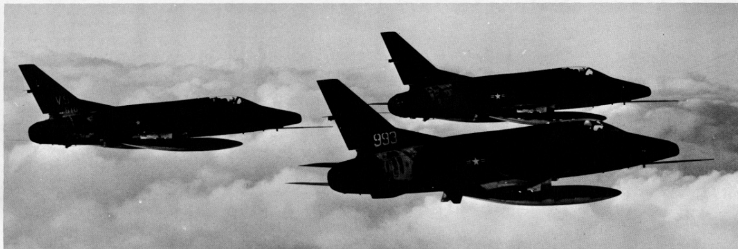
Supersonic air warrior: The first fighter to attain level supersonic flight, the F-100 was North American's improvement on the F-86 design, an evolution mandated by the Soviet MiG-15's ability to fly higher and outclimb, outturn and outaccelerate the Sabre in the Korean War.
