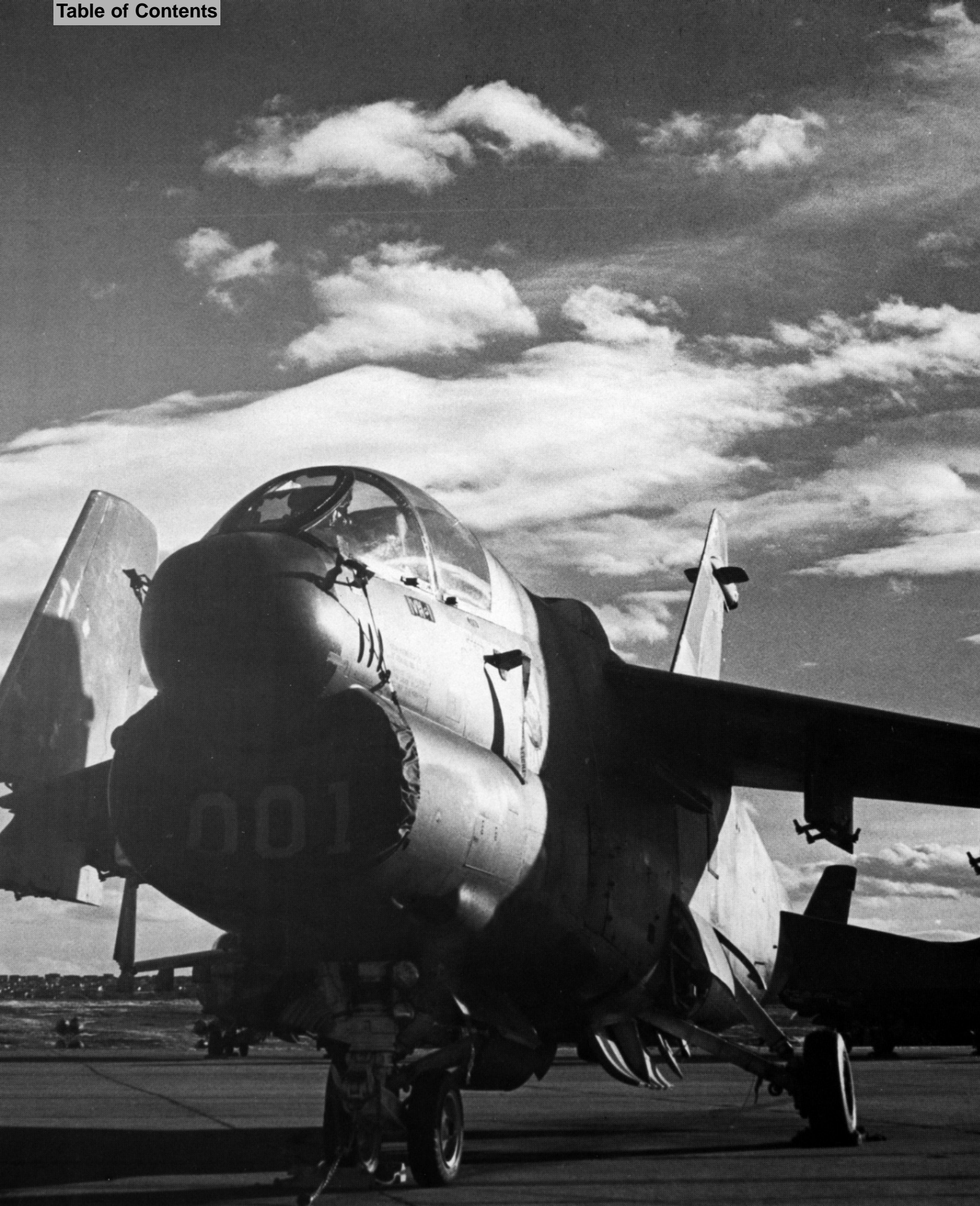
Corsair II: The A-7 is the third Vought aircraft to carry the Corsair nom de guerre. Developed as a result of the Navy's Sea Based Strike Study in the 1960s, even the Air Force version of the Corsair sported foldaway wings.
